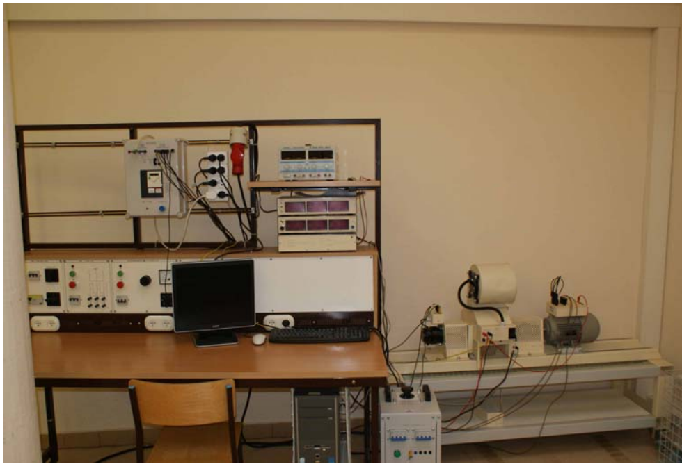
Rys. 4. Laboratory stand for testing cage motor
