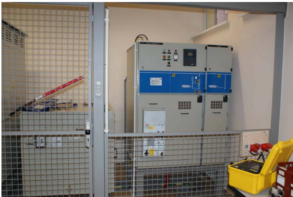
Rys. 7. The laboratory stand of HV (15 kV)
