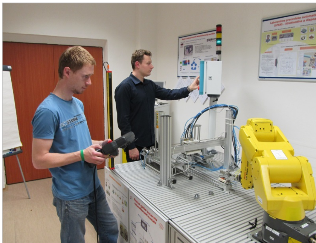
Fig. 3. Fanuc robot online programming
